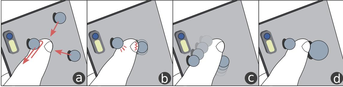
**Figure 2: The stimuli dimensions of Pulp Friction illustrated at the back of a phone. (a) Marbles coming to poke the finger from different angles. The left marble is rolling beside the finger describing a *pattern*. (b) Marbles poking and vibrating beside the finger resulting in different *sharpness* of stimuli. (c) Marbles rolling beside the finger at different *speeds*. (d) Marbles of different *sizes* contacting the finger periphery.**
