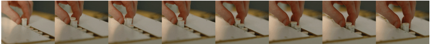
Figure 1. A sensel-based slider control, as used in the studies reported here. As the user tilts the sensel and moves their grasp from one raised rod to the next, adjacent components rise and fall on-demand to give the impression—and feeling—of moving a tangible slider thumb along a static guide rail.
