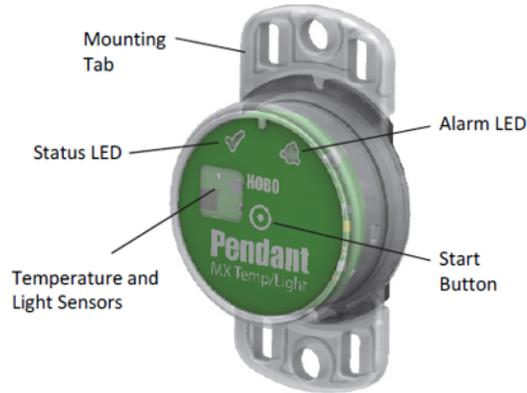
**Figure 1:** The Onset MX2202 HOBO Pendant MX Temperature, Water Temperature and Light Intensity Data Logger
