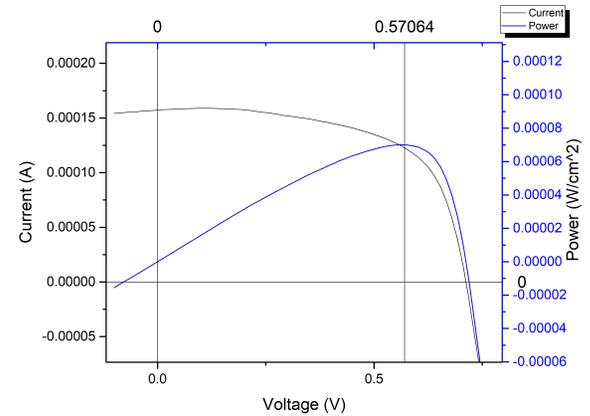
**Figure 4:** An example data set acquired from the candlelight ageing MPPT using the scenario from an office scenario with some incident natural light for an inverted (PIN) structure PSC.
