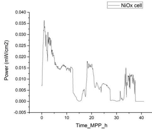
**Figure 3:** An example data set acquired from the candlelight ageing MPPT using the scenario from an office with partial incident natural light for an inverted (PIN) structure PSC.
