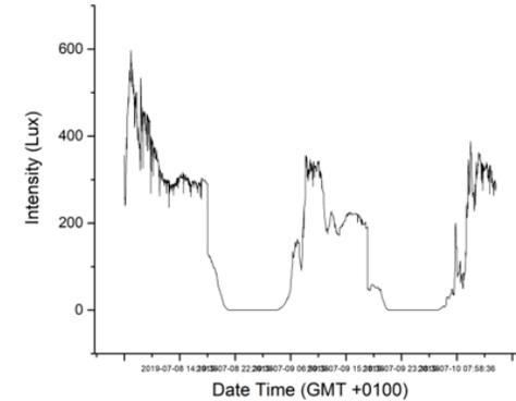
**Figure 2:** An example data set acquired using the data logger from an office scenario with some incident natural light
