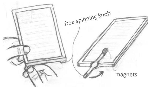
Figure 1: An E-book that only stores one digital book. Rotating the handle 180 degrees will generate the energy to 'flip' to the new page, and thereby acts as an input.
