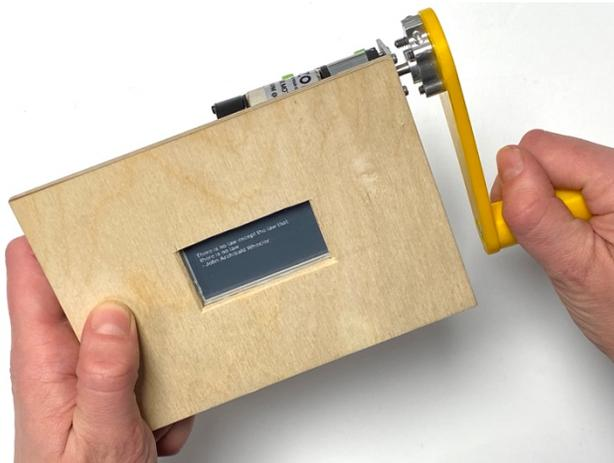
**Figure 1:** The hand cranked quote reader made to explore the design of HPIS. The machine allows scrolling back and forth through 20 famous science quotes. The quotes stay on screen after cranking since we used an e-paper display. The machine also preserves its state between cranks.
