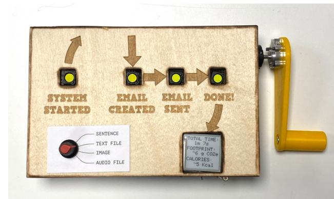
**Figure 2:** The human-powered email machine exploring hand cranked communication. The user boots the system by cranking until the magnetic indicator shows that the system has started and then can choose to send 4 different sized emails. After selection users have to crank through the progress bar until done and the e-paper display shows total time and estimations for saved carbon footprint and burned calories.
