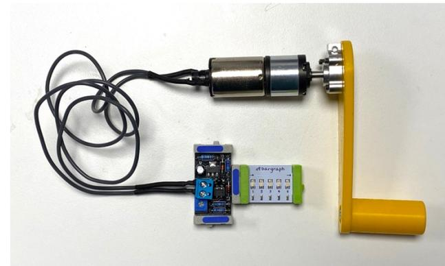
**Figure 4:** The Human-powered LittleBit connected to a DC motor with a 1:104 gear ratio. The power only snap connected to a bargraph which serves as an easy way to explore the difference between the three output snaps.
