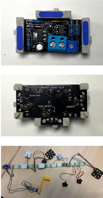
**Figure 3:** The human-powered LittleBits based on the Peppermill circuit. The top 2 images showing front- and backside of the LittleBit. The LittleBit has three output snaps. The middle output provides only power. The left snap both power and the direction of cranking on the signal line. The right snap provides an adjustable speed of the cranking. The bottom image showing a typical exploration made by a student group with various sensors and actuators.
