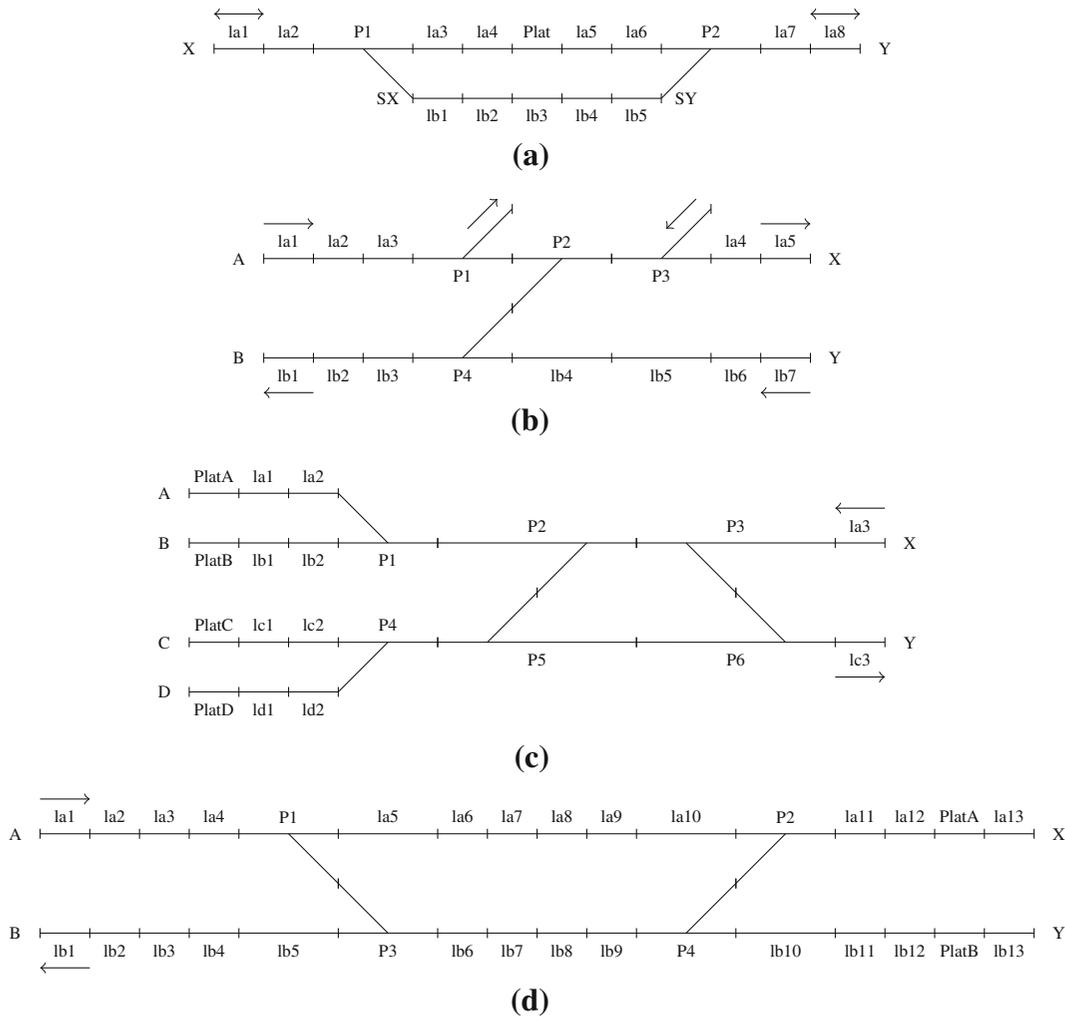
**Fig. 13** Verified track plans. **a** A pass through station (TP-A), **b** a double junction (TP-B), **c** a terminal station (TP-C), **d** a modified track plan from a London Underground station (TP-D)
