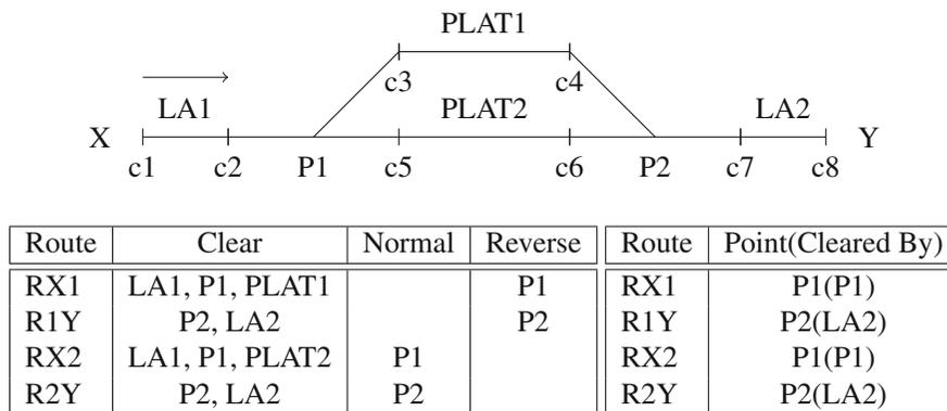
**Fig. 4** A scheme plan for a simple station. *Top* track plan, *bottom left* control table, *bottom right* release table
