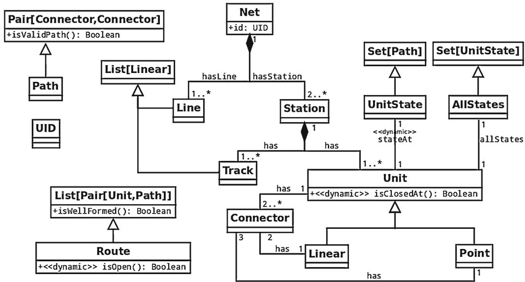
Fig. 1 Part of Bjørner's DSL captured in a UML Diagram
