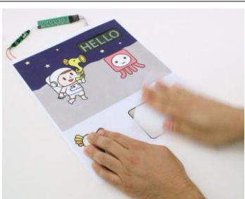
Figure 2. Paper Generator harvests energy from rubbing and activates the e-paper display, revealing the word "hello" [5].
