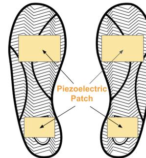
Figure 1: Figure 1. Piezoelectric Patch under shoes design
