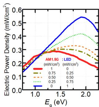
Figure 3: Estimated electrical power density generated at a constant optical power input of 1 mW/cm<sup>2</sup> for different ratios of AM1.5G sunlight and LED illumination.
