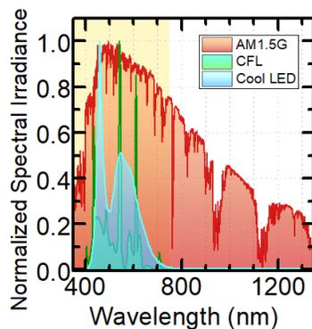
Figure 1: Normalized spectral irradiance of sunlight, CFL and LED light sources.
