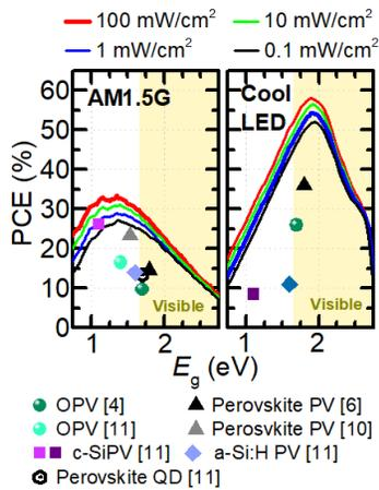
Figure 2: Theoretical limit of the PCE as a function of the PV's bandgap for sunlight with a standard AM1.5G spectra and a cool LED spectra with various irradiance values. Symbols are the experimental PCE values reported in the literature and certified by NREL for some emerging PV technologies and for c-Si and a-Si:H PV.
